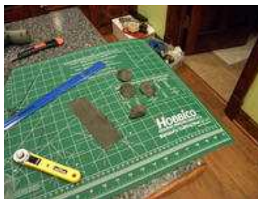
Lay them approximately centered over the bolt holes Wet them out with thin CA
